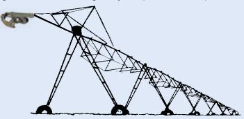
APPLICATION: Install at the end of center pivot systems for automatic flushing at start-up and shut-down — or, configure with an electric solenoid interfaced with the center pivot for automatic flushing while system is operating.
